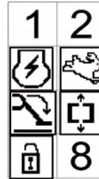
Fig. 148 Emergency BY-PASS activated
