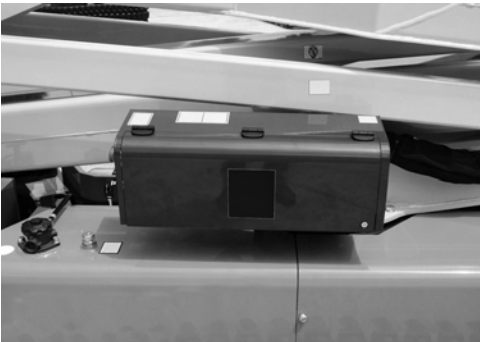
Fig. 124 Aerial part distributor protection
