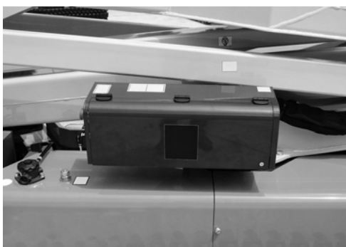
Fig. 136 Aerial part distributor protection
