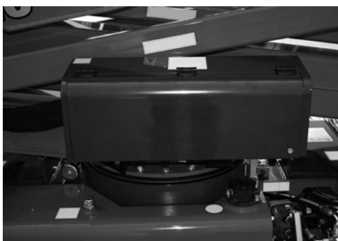
Fig. 123 Aerial part distributor protection
