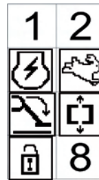
Fig. 130 Emergency BY-PASS activated
