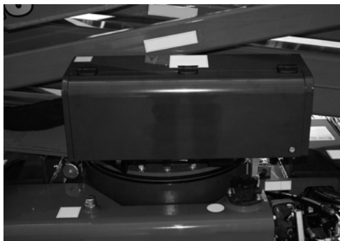
Fig. 111 Aerial part distributor protection
