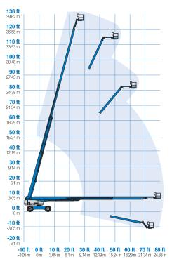
$^{\ast}$  The metric equivalent of working height adds 2 m to platform height. U.S. adds 6 ft to platform height.
