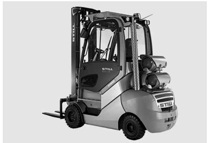
Driver's cab set high for an improved all-round view
