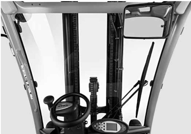
Narrow profile of protective roof and mast optimises forward visibility
