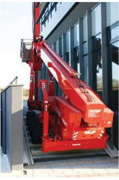
The outriggers and automatic levelling system allow the operator to set the Spider up on different levels. This is needed as the Spider is being set up on the steps of the grandstand. The easy-to-use controls with colour coded functions also make the Teupen Leo 36T very user-friendly.
